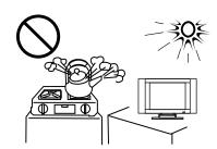
The vents and other openings in the cabinet are designed for ventilation. Do not cover or block these vents and openings since insufficient ventilation can cause overheating and/or shorten the life of the product.
